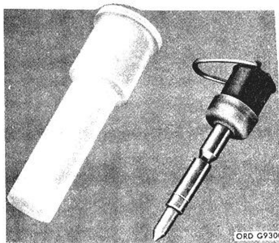
Figure 43. Explosive cartridge and case.
